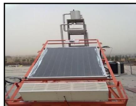
*Thermal Performance Test Set-up*
